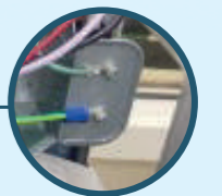
Separate earthing for PCBs
